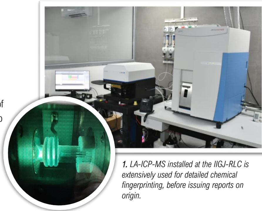
1. LA-ICP-MS installed at the IIGJ-RLC is extensively used for detailed chemical fingerprinting, before issuing reports on origin.
