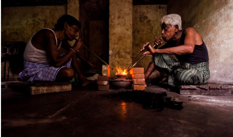
Treaters practicing the ancient art of blowpipe heating in Ratnapura, Sri Lanka. As described by al Beruni ca. 1045 AD, the temperatures reached by this technique exceeds that of the melting point of gold (1064°C). From Hughes et al., 2014 . Photo: Wimon Manorotkul, 2012. Click on the photo for a larger image .
