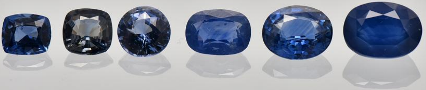
HT+P treated sapphires. Photo: SSEF. Click on the photo for a larger image.
