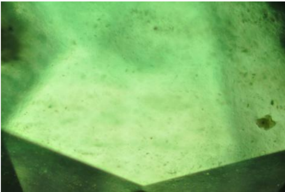
Figure 3: Most of the Jharkhand emerald appeared hazy due to presence of minute mineral inclusions. Magnified 32x
