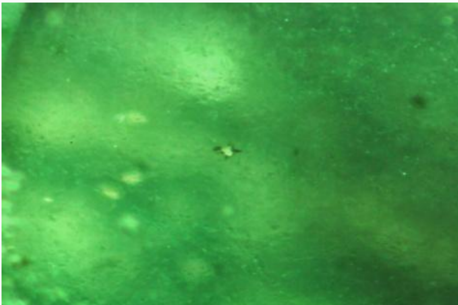
Figure 7: Zircon-Halo was the most striking inclusion seen in these emeralds, which were never seen before in emeralds. Magnified 80x
