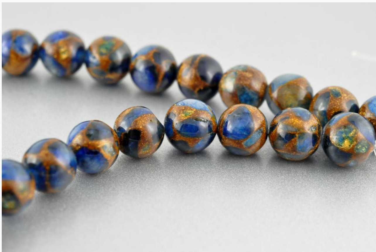
Figure 1: This string weighing 145.70 carats consists of attractive blue and golden brown beads measuring approximately 7.91–8.48 mm in diameter. The beads were identified as composites fashioned from pieces of dyed quartzite held in a polymer matrix.
