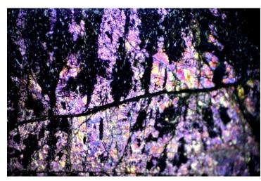
**5.** The 44.31 ct cabochon of heterosite-purpurite displayed fine layered structure, responsible for strong sheen and iridescence. Black intermittent areas are mineral grains (also heterosite).
