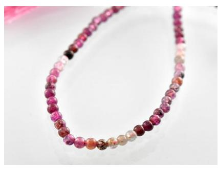
**14.** This string containing beads of corundum (ruby and sapphires) was proved to be fissure-filled with resin, by infrared spectroscopy.
