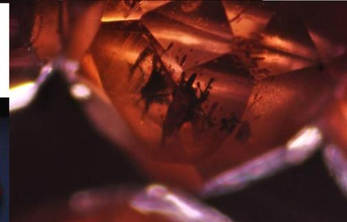
3. Black-opaque inclusions are a common feature in HPHT-grown synthetic diamonds, which were present in these beads also.
