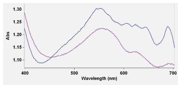
10. UV-Vis-NIR spectra of violet beryl displayed a typical pattern associated with 'maxixe-type' beryl with a series of bands in the region 500-700 nm (blue trace – 'o' ray).
