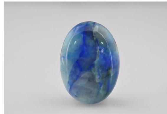
7. This 16.31 ct cabochon was identified as potassium feldspar coloured by azurite within the fissures.
