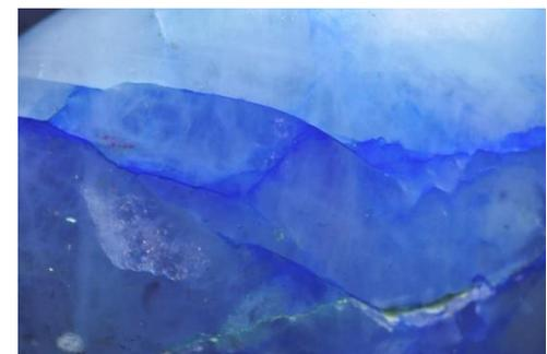
8. Fissures with blue material (azurite – identified by Raman spectra) were relatively wide, which suggested that these are rather natural.
