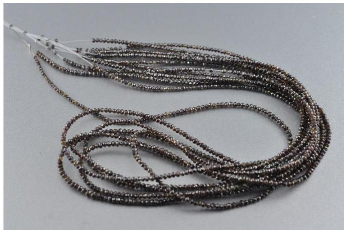
1. Red-brown beads in this bunch, weighing 79.28 ct were identified as HPHT-grown synthetic Type-Ib diamonds.
