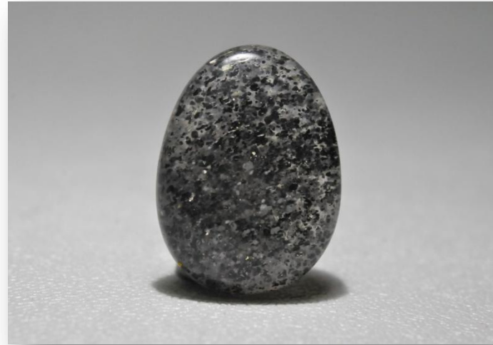
10. This 23.61 ct specimen of quartz was interesting because of abundant black graphite inclusions.
