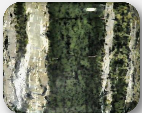
6. This 45.25 ct banded serpentine is composed of green antigorite and pale yellow chrysotile. Also note the sheen effect in chrysotile portion, caused by parallel fibrous structure.
