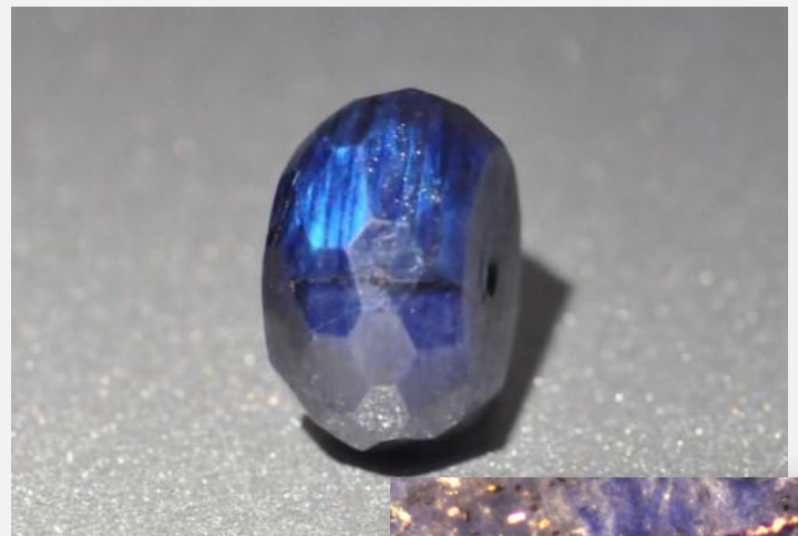
Figure 7: This 3.73 ct bead was proved to be dyed labradorite. Note the strong blue labradorescence and colour concentrations in fractures (right)
