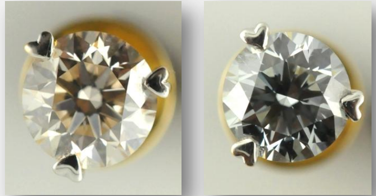
Figure 8: This synthetic CVD diamond changes colour from light brown (left) to light grayish blue (right) on exposure to shortwave UV, and regain the original colour on exposure to a filament lamp
